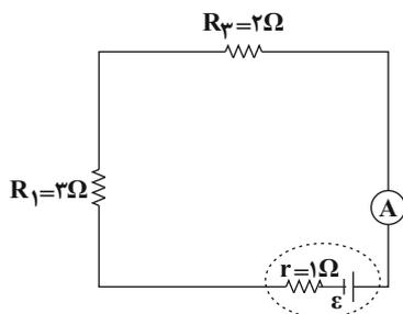
$$R_{eq} = R_1 + R_3 = 3 + 2 \Rightarrow R_{eq} = 5\Omega$$
